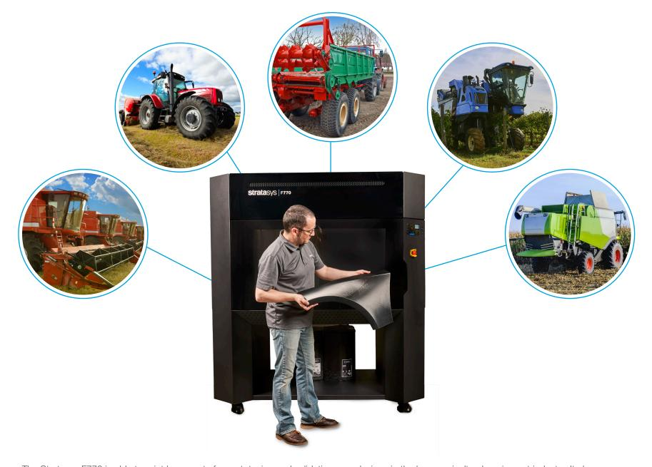
The Stratasys F770 is able to print large parts for prototyping and validating new designs in the large agricultural equipment industry. It also offers an economically viable means for end-use parts either as a bridge to full production or to produce low volumes of out-of-production parts.
